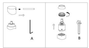
**Cleaning of Aerator** To avoid the dust and impurities from construction that might influence the water flow, it is suggested to clean the aerator on a regular basis.
